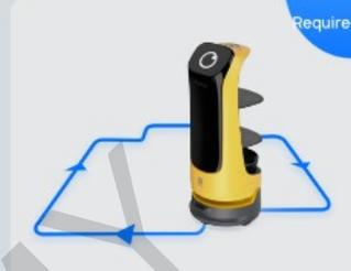
The robot circulates along a predetermined path in Cruise and Customer Attraction
