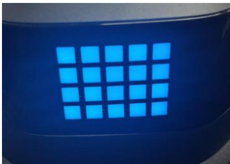
Power on — All indicator lights turn on
