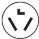
3-wire receptacle (10-30R)
