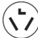
3-wire receptacle (10-30R)
