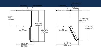
Allow door swing clearance at locations next to a wall. If the appliance is installed with the hinges next to a wall, the distance between the appliance and the wall must be at least  $1\,\%$ " (40 mm). This is how far the handle protrudes when the door is open. The refrigerator door must open to a minimum of 90° to allow the crispers to open and the shelves to be removed. A 90° door limiter is available for this model. Height can be increased by 3/8" (10mm) by turning the levelling feet at the
