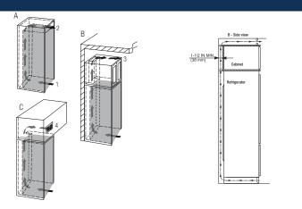
If the appliance is integrated in a fitted kitchen, the following ventilation requirements must be met: - The spacing fins on the back of the appliance are used to ensure sufficient ventilation. These must not lie in cavities or recesses in their final installation position. - Basically, the larger the ventilation gap, the more energy the appliance saves during operation. Do not restrict the air flow.
