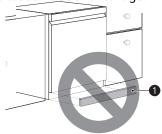
Remove the protective film from the door, if present. Leaving the film on may cause discoloration or condensation on the door.
