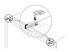
Bend the tabs on the brackets to secure them to the frame using a pair of needle nose pliers.
