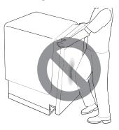
· Do not push the top of the dishwasher. Doing so can damage the interior of the dishwasher.
