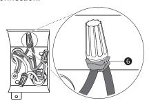
**10** Fold the connected wires back into the junction box and screw on the junction box cover.
