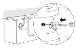
Remove the knockout plug 1 from the disposal.
