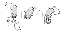
Remove any debris with a brush, if needed. The cover can be cleaned under running water. Allow it to dry before reassembling it to prevent water from entering the blower tube.
