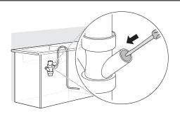
Attach the drain hose to the waste tee with the hose clamp provided. Move the clamp into position and tighten it with a flat-blade screwdriver.
