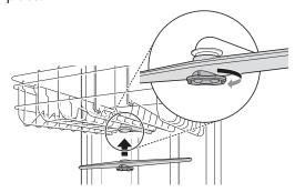
After assembly, make sure that the spray arms rotate freely.
