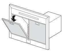
• To reassemble the filter, insert the back of the filter first and then lift the filter up into place.
