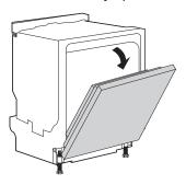
Use the door adjustment screws provided to adjust the door spring tension at the bottom of the dishwasher.
