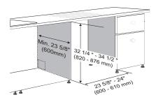
To allow for proper clearance of plumbing and electrical, use the template included with the literature to determine the clearance on the side of the cabinet where the cabinet meets the back wall. Using a 2 1/2" diameter hole saw, drill a hole in the target area as shown on the template.
