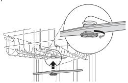
7 After assembly, make sure that the spray arms rotate freely.
