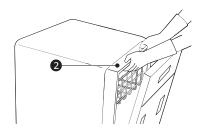
Align the dishwasher with the opening. Make sure the water supply line and power cord kinks or bends.
