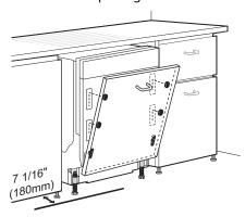
Attach the cabinet panel to the dishwasher door on the sides using the provided bracket screws.
