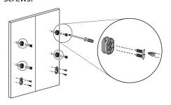
Attach the lower panel brackets (provided) to the cabinet panel using the provided wood screws.
