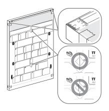
Use a 1/16" (2 mm) diameter drill bit to drill 3/ 8" (10 mm) deep pilot holes at the 12 points marked on the template.
