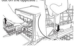
To remove the back rack supports from the rails, hold a side rail with one hand, lift the front of the rack, and firmly push the rack
