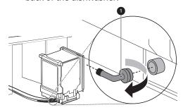
**2** Connect the water supply tube to the elbow.
