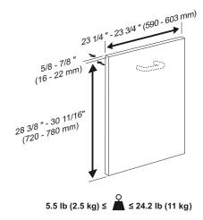
For best results, the width of the wood panel should be 1/4" (6 mm) less than the width of thecabinet.
