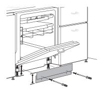
Attach a custom toe kick. If needed, use a saw to cut a notch in the top of the custom toe kick to provide clearance for the cabinet panel when opening the door.
