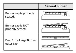
To assemble the dual extra large burner outer cap properly, make sure that the burner cap **1** is positioned over the assembly guide **2** in the burner head.
