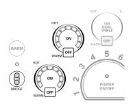
2 Select a number in the element power settings to adjust the power level. If a power level is not selected after 10 seconds, the element's power level remains the same.
