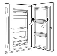
2 To replace the door bins, slide the door bin in above the desired support and push down until it snaps into place.
