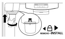
**5** After the water filter is replaced, dispense 2.5 gallons of water (flush for approximately 5 minutes) to remove trapped air and contaminants from the system.
