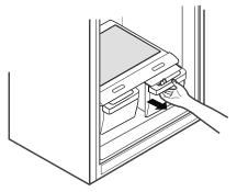
**2** To reassemble, slightly tilt up the front of the crisper, insert it into the frame, and push it back into place.
