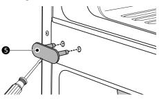
8 Remove the decorative screw **6** located on the housing between the freezer and refrigerator doors. (You will need this hole for the middle hinge bracket.)
