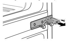
Using a 1/4 in. socket wrench, loosen and remove the bottom hinge pin 4 from the bottom hinge bracket 5. Remove the washer from the bottom hinge pin and set it aside.
