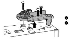
6 Move the bracket to the opposite side of the door and insert the hinge pin sleeve. Reverse the hinge lever ④ by flipping it over. Place it on top of the bracket, and tighten both down with the screw. Then insert the remaining 2 screws to tighten the bracket to the refrigerator door.
