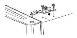
**2** Place the top hinge on top of the freezer door and line up the hinge with the holes on top of the refrigerator. Use the three bolts to fasten the hinge.
