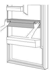
**2** To assemble the bin, slide it in above the desired support and push down until it snaps into place.
