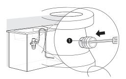
**2** Remove the knockout plug **1** from the disposal.
