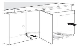
**5** Remove the tape from the water supply line and the electrical cable.
