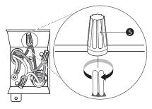
**9** Wrap electrical tape **()** around each connection.
