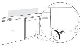
3 Use a Phillips screwdriver to remove 2 screws **①**.
