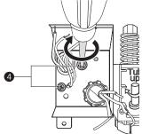
8 Pair the white, black, and green wires to the matching colored wires from the dishwasher. Then twist on the provided wire nuts **S** tightly to connect the corresponding wires.
