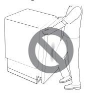
• Do not push the top of the dishwasher. Doing so can damage the interior of the dishwasher.
