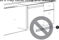
Remove the protective film from the door, if present. Leaving the film on may cause discoloration or condensation on the door.
