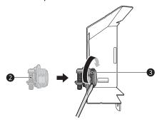
**6** Insert the electrical cable through the hole in the strain relief. Tighten 2 screws to secure the cable.
