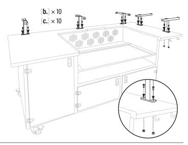
**STEP 03** Use ten (10) 1/4"x1" bar counter bolts [**b**.] and ten (10) 1/4" bar counter lock nuts [**c**.] to attach the long and short bar counters to the bar supports.
