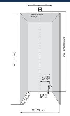
The appliances can be used freestanding or semi built-in. If semi built-in, consider the minimum cabinet opening dimensions specified on this image.
