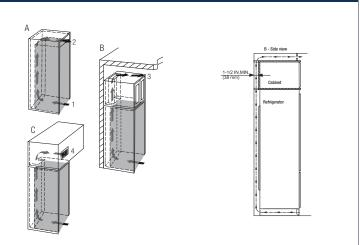
If the appliance is integrated in a fitted kitchen, the following ventilation requirements must be met: - The spacing fins on the back of the appliance are used to ensure sufficient ventilation. These must not lie in cavities or recesses in their final installation position. - Basically, the larger the ventilation gap, the more energy the appliance saves during operation. Do not restrict the air flow.
