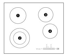
The cooking zones have maximum power available to them. If this power range is exceeded by using multiple cooking zones simultaneously, power
