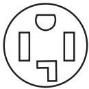
4-wire receptacle (14-30R)
