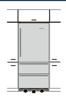
CS 20 appliances don't need any ventilation openings in the cabinet. The required airflow is directed through the toe kick area.
