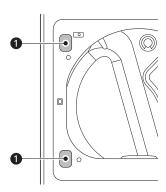
2 While supporting the door, remove the 2 screws 2 on the door hinge, two from each hinge. Set the door aside face down on a protected surface to prevent damage to the door or the work surface.
