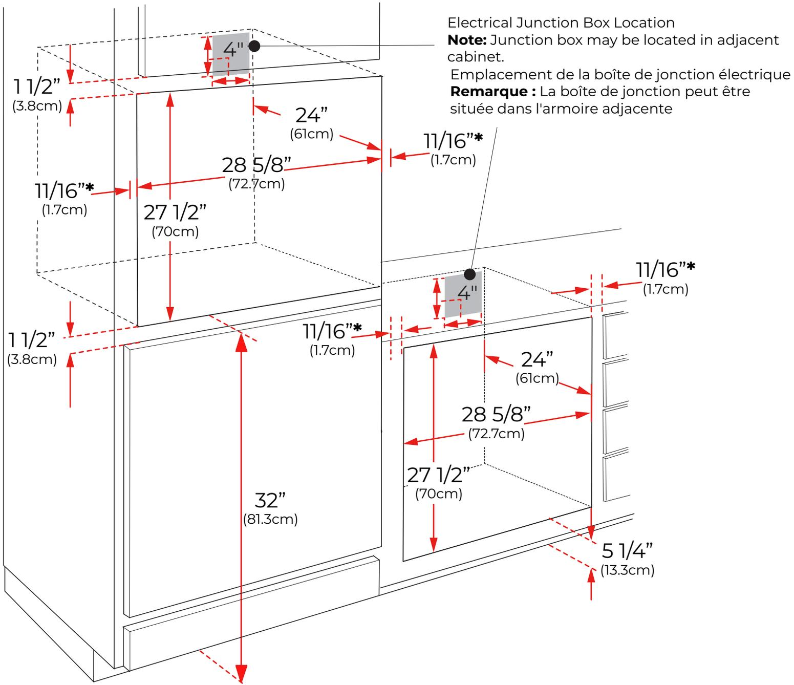
**\*The 11/16" measurement indicates the overlap of the oven sides with the cutout.
