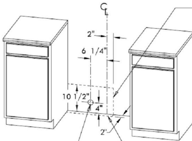
Area allows for flush installation with through-the-wall connection of pipe stub/shut-off valve and rear wall 110/120V outlet.
