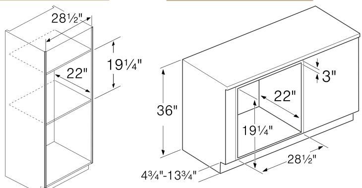
**NOTICE:** The cabinet base must be flat and capable of supporting a weight of at least 142 lbs (64.1 kg).
