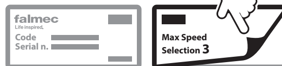
Fig. 1: Set maximum speed 3:
