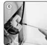
Install water valve on refrigerator cabinet with screw.
