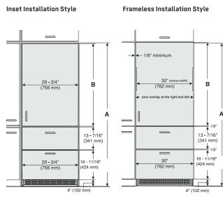
Product also allows installation with Toe kick height of 2" (50mm) to 6 11/16" (170mm). To define the panel height other than 4" (102mm) toe kick, consider 20 11/16" (526mm) - toe kick height
