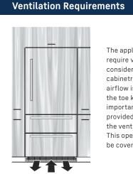
The appliance do not require ventilation considerations in the cabinetry. The required airflow is directed through the toe kick base. It is important to use the provided cover grille for the ventilation opening. This opening must not be covered.
