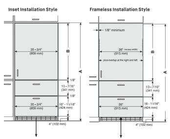
The height of this panel cannot be reduced for higher toe kicks as it will reveal structural elements of the appliance. Instead, install appliance on a platform and adjust the opening height to accommodate.
