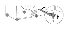
5.2 Attaching the spacers to the dryer.
