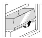
2 To assemble drawers, slightly tilt up the front, insert into the frame and push back into place.
