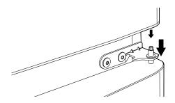
Place the top hinge on top of the freezer door and line up the hinge with the holes on top of the refrigerator. Use the three bolts to fasten the hinge.
