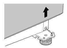
**3** Loosen the 2 bolts and remove the middle hinge bracket from the refrigerator housing. Set the parts aside.
