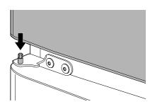
Place the top hinge on top of the freezer door and line up the top hinge with the holes on top of the refrigerator. Use the three bolts to attach the hinge.
