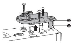
Move the bracket to the opposite side of the door and insert the hinge pin sleeve. Reverse the hinge lever 4 by flipping it over. Place it on top of the bracket, and tighten both down with the screw. Then insert the remaining 2 screws to tighten the bracket to the refrigerator door.
