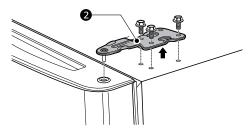
**3** Lift the freezer door slightly and remove it.
