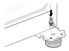
**6** Using a 3/8 in. socket wrench with a 2-inch extension, loosen the 3 bolts on the bottom hinge bracket.
