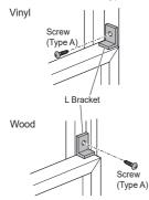
Remove the screw from the bottom right of the cabinet. Attach the support bracket using the screw you just removed. Secure the support bracket to the inner window sill using a type B screw.
