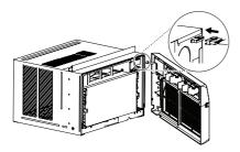
Remove air filter from the front grille by pulling the filter forward and then up slightly. Secure it with 2 type A screws through the front grille.
