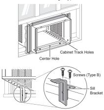
3 Carefully place the cabinet back in the window and align the cabinet track holes with the support brackets. Attach each support bracket to the cabinet through a cabinet track hole, using a type D screw and a lock nut. Use the first track hole past the sill bracket on the outer edge of the window sill. Tighten the lock nuts on the support brackets to secure them to the sill brackets.
