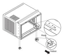
5 Insert the top and bottom rails of the curtain panels into the upper and lower panel guides.
