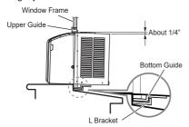
Extend the guide panels to fill the window opening and use 2 type B screws and 2 type C screws to secure them to the window.
