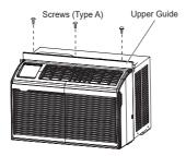
Insert the top and bottom rails of the curtain panels into the upper and lower panel guides Fasten the curtain panels to the unit with 8 type A screws Fasten screws behind the curtain panel.
