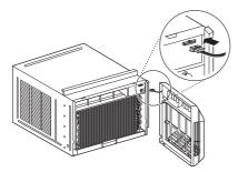
5 Attach the front grille to the cabinet by inserting the tabs on the grille into the slots on the front top of the cabinet.
