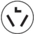
3-wire receptacle (10-30R)
