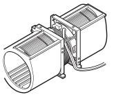
Rotate and reinstall the blower unit ① so that the exhaust ports ② face the rear of the cabinet and are aligned with the rear knockouts. When you insert the blower unit, the blower wire ③ must be routed as shown.
