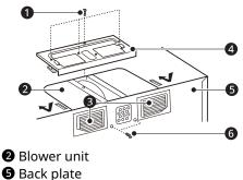
7 Insert the tabs on each side of the damper into the holes at the inside rear of the adapter. Attach the exhaust adapter ① to the back plate wall side. Push in securely until it is past the top locking tabs ③ and in the lower locking tabs ③. Make sure that the damper hinge is at the top and that the damper swings freely.
