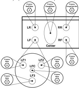
To prevent leakage, make sure the orifice spuds are securely screwed into the gas supply tubes.
