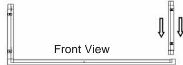
4. Locate top panel and align with top of right and left side panels. Fully insert top panel into right and left side panels until locking tabs lock completely.
