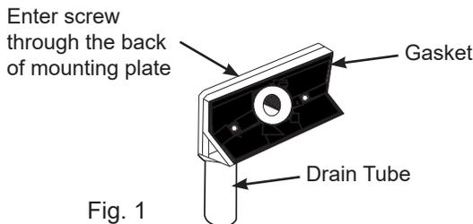
2. This assembly may now be installed into either the left or right drain holes on the rear flange of the sleeve, using two (2) of the screws (Type A for Metal cabinet or Type B for Molded) included.
