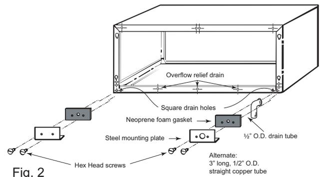
4. A tube or hose 1/2" I. D. (obtained locally) may be installed onto the drain tube to drain any overflow water away from the installation (to a gutter or the ground).
