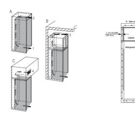
If the appliance is integrated in a fitted kitchen, the following ventilation requirements must be met: - The spacing fins on the back of the appliance are used to ensure sufficient ventilation. These must not lie in cavities or recesses in their final installation position. -Basically, the larger the ventilation gap, the more energy the appliance saves during operation. Do not restrict the air flow.
