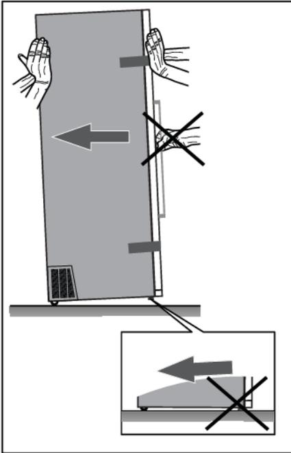
When moving the appliance, be careful not to push it on the floor because of potential damages. There are two casters on the back of the appliance housing, that make moving the appliance around easier.
