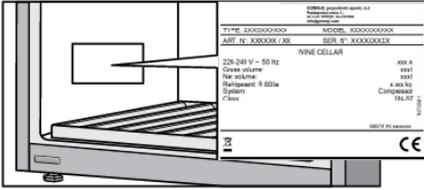
Place the appliance in a dry and well aired room. The permitted ambient temperature range for the appliance depends on the appliance's climate class, which is shown on the type plate.
