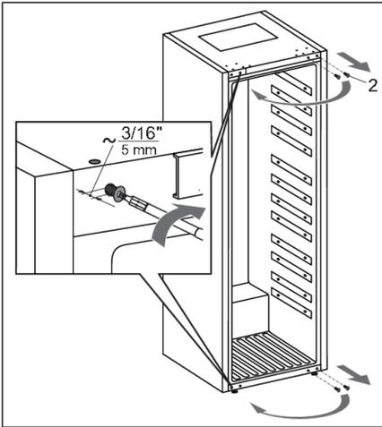
8. Completely undo the screws (2). Then, partly screw them into the holes at the top and bottom on the opposite side of the housing.
