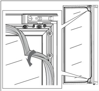
2. Release the screws (1) at the top and bottom. Do not undo them completely!
