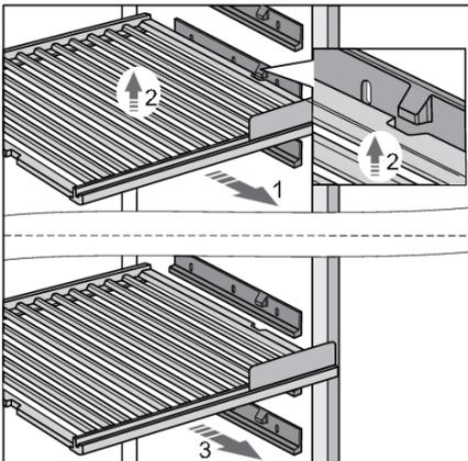
To remove a shelf from the appliance, partly pull it towards you (1) until the two grooves on the shelf and the block on the plastic shelf supports are aligned. Then, lift the shelf (2) and pull it out from the appliance (3). Take care not to damage the door gasket.
