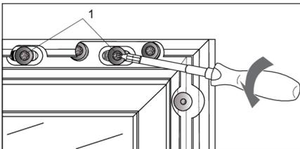
3. Close the door, then rotate the screw (2) at the top and bottom to adjust the door position.
