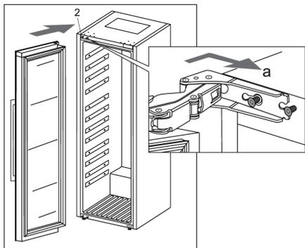
10. Hang the door onto the screws (2) at the top and bottom and slide it in the direction indicated by the arrow (a).
