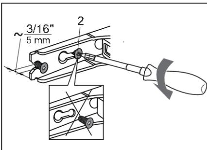
3. Partly (by no more than 5 mm) undo the hinge screws (2) at the top and bottom. Do not completely undo the screws. This way, the door will remain in contact with the housing.
