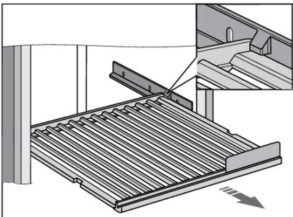
The shelf can also be partly pulled out from the appliance. The blocks on the plastic shelf supports protect the shelf from being fully extended and pulled out, which could result in the shelf falling from the appliance.
