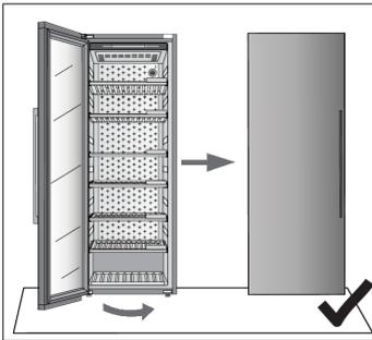
15. Close the door and make sure it is aligned with the housing. The housing side and the edge of the door should be parallel.
