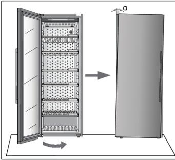
If the door is not aligned with the housing (the angle  $\alpha$  is not  $0^\circ$ ),
