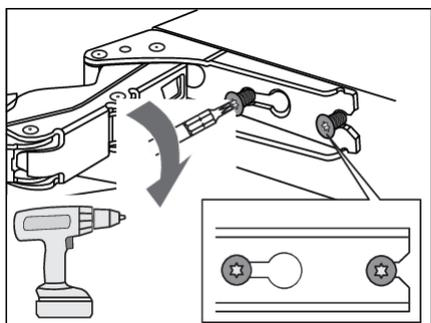
11. Tighten the screws. The screws should be tightened to a torque of 6.2 Nm.
