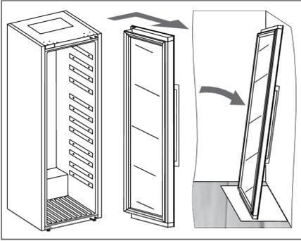
4. Remove the door, complete with the hinges, by moving it in the direction indicated by the arrow. Carefully place the door on the surface prepared for this purpose.
