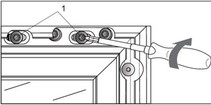
5. When the door edge is parallel to the housing side, open the door again and tighten the screws (1) you released at the start of the door adjustment process.
