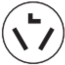
3-wire receptacle (10-30R)
