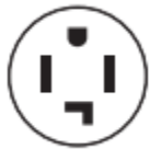
4-wire receptacle (14-30R)
