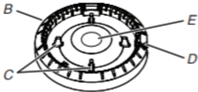
A. Burner cap B. Burner base C. Alignment pins D. Igniter electrode E. Gas tube opening
