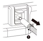
**2** Connect the drain hose of the dryer and secure the hose clamp.
