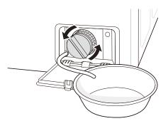
**5** Clean the pump filter and opening.
