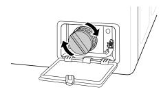
**8** Close the drain pump filter cover.
