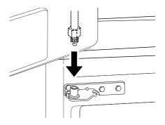
2 Fit the hinge **1** over the hinge lever latch **2** and slot it into place. Rotate the lever **3** clockwise and fasten the hinge.
