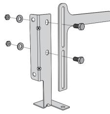
3. Align the base of the hook of the bracket with the base on the slot of the rear wall fastening bracket. Align the base of the fastening bracket with the floor and tighten the screws to fix the measurements.
