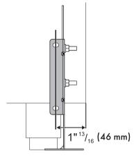
6. Move the bracket to the wall and fix with the two washers and screws. A qualified technician must verify the suitability of the materials in accordance with the type and condition of the wall.
