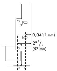
After having positioned and leveled the appliance, move the bracket close to the rear of the appliance and anchor it to the floor using the two washers and screws. A qualified technician must verify the suitability of the materials in accordance with the type and condition of the floor.
