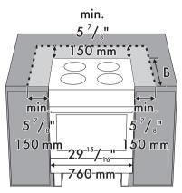
The side cabinet depth (clearance **B**) must match the front edge of the range side panel.
