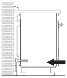
Check for proper installation and use of the anti-tip bracket. Carefully tip the range forward by pulling it from the back to ensure that the anti-tip bracket engages the range leg and prevents tip-over. The range should not move more than 1" (2.5cm).
